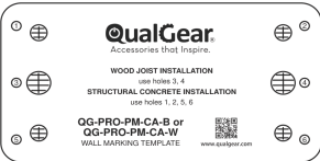
Wall marking template
